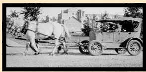
Bennett buggy: a term used to describe a car which had its engine and windows taken out and was pulled by a horse.
